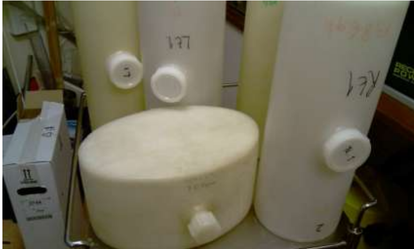
Figure 7.1 - containers used for body phantom
