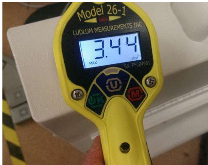
Figure 3.1c - follow up dose rate checks on ^{57}\text{Co} package
