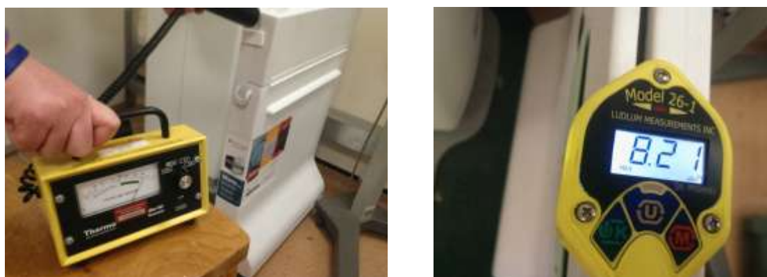
Figure 3.1b - contamination and dose rate monitoring of ^{57}\text{Co} source package
